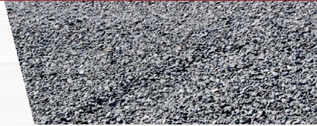
4-6" crushed limestone recommended for the pad
